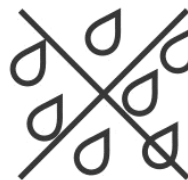
FIG. 4 LAMP TO BE USED IN DRY CONDITIONS OR IN A LUMINAIRE THAT PROVIDES PROTECTION
