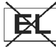
FIG. 5 LAMP NOT SUITABLE FOR EMERGENCY OPERATION
